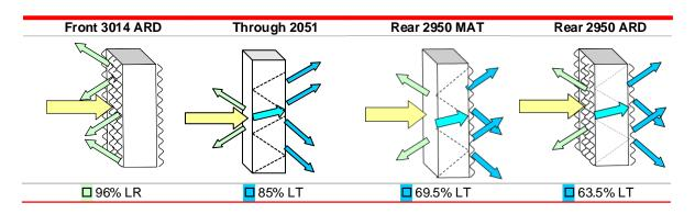
Values of light transmission/light reflection for a standard in 4 mm.
