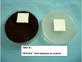
Same tests have been done after thermoforming to ensure the efficiency of the material. Please notice that protection is reduced a bit due to the significant reduction in thickness (samples tested after thermoforming where 0.6-0.8mm thickness).
