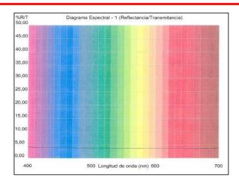
Reflectance spectrum in visible range for CRYLUX<sup>™</sup> 3945 in 3 mm thickness
